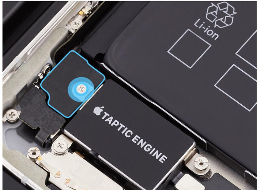
3. Use ESD-safe tweezers to remove the Taptic Engine cowling. Save the cowling for reassembly.
