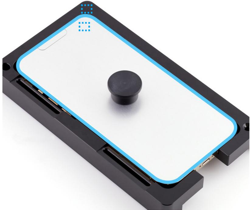
7. Position the repair tray with the iPhone in the display press. Pull down the lever until the display press locks.
