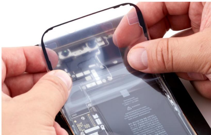
6. Place the display adhesive press plate on top of the enclosure with the icon in the top right corner as shown.
