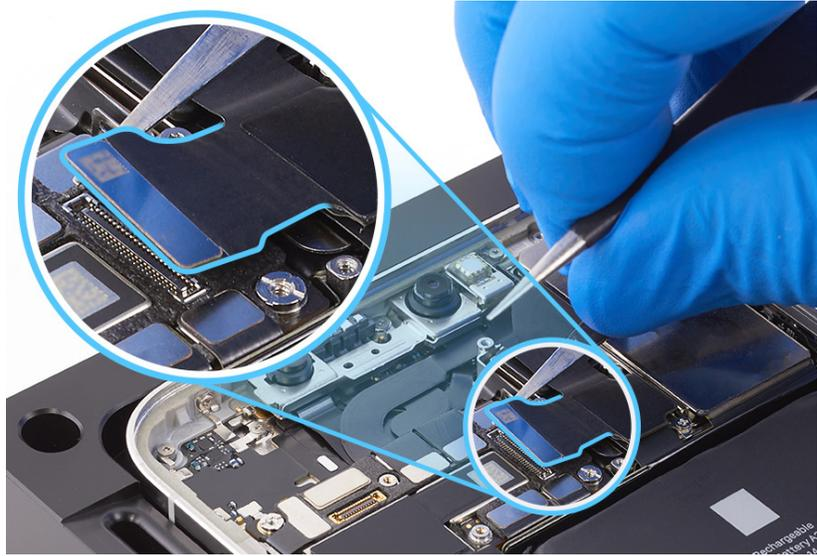
5. Use ESD-safe tweezers to lift the end of the bottom camera flex cable off the connector.
