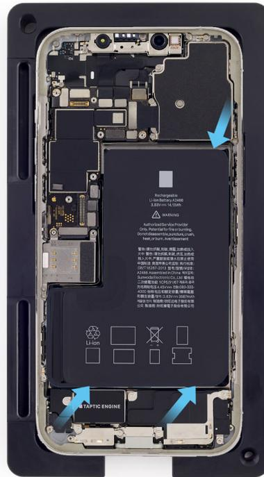
15. Slightly lift the battery with the black stick just enough to grasp underneath the battery.
