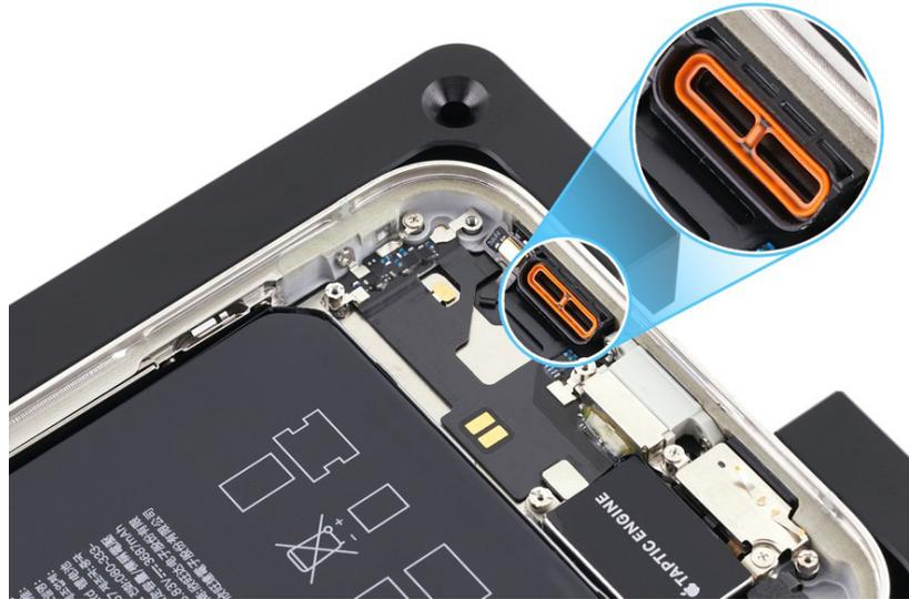
2. Ensure that the speaker foam is intact and the grounding springs on the speaker aren't bent or broken.
